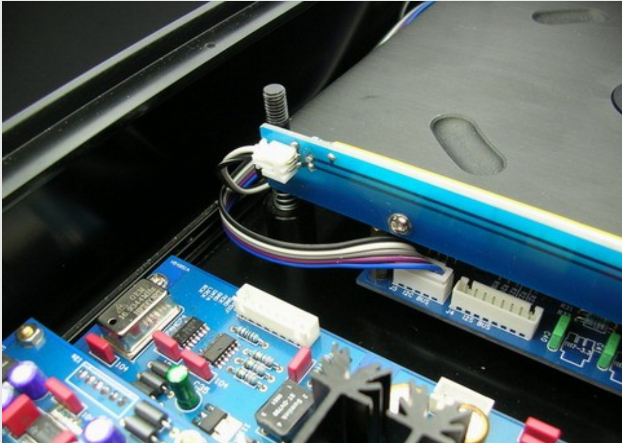
Connect wire from Display Board to Laser Pickup Module
