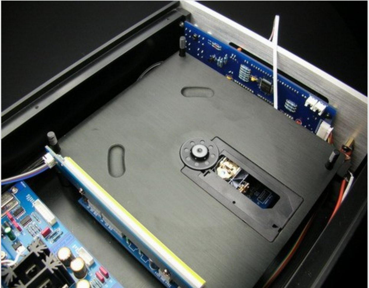
Connect wire from Display Board to Laser Pickup Module
