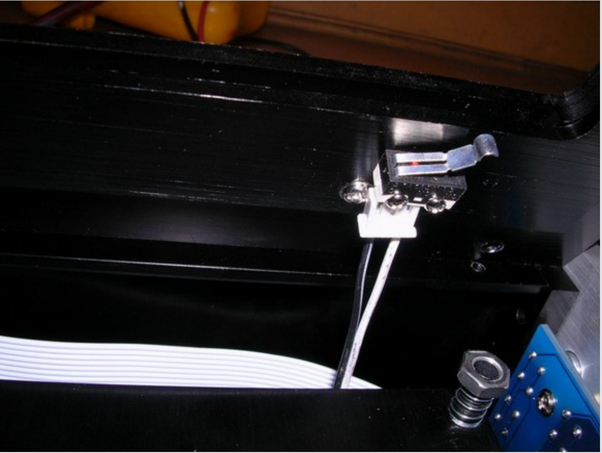
Connect Top cover switch cable and install Top cover
